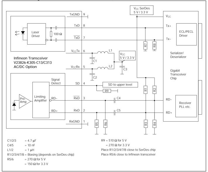
Values of R1/2/3/4 may vary as long as proper 50  $\Omega$  termination to  $V_{EE}$  or 100  $\Omega$  differential is provided. The power supply filtering is required for good EMI performance. Use short tracks from the inductor L1/L2 to the module  $V_{CC}Rx/V_{CC}Tx$ .
